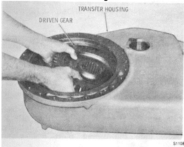
Fig. 6-90. Removing front bearing from transfer housing
