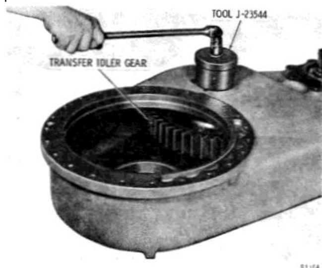
Fig. 6-87. Removing transfer idler gear spindle.
